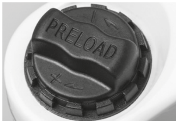
Figure 29: Negative deflection setting wheel on the suspension fork crown
