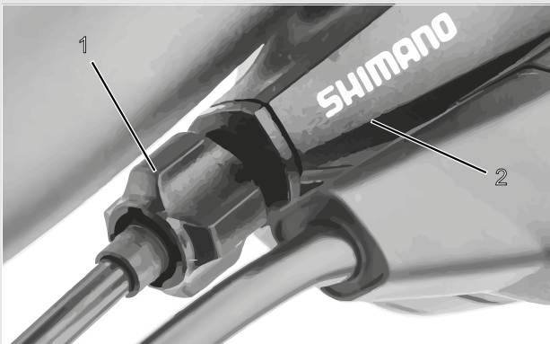
Figure 43: Adjusting sleeve (1) for the single-cable, cable-operated gear shift with shifter housing (2), example
