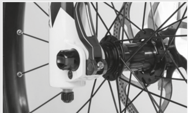
Figure 41: Adjusting the quick release clamping force
