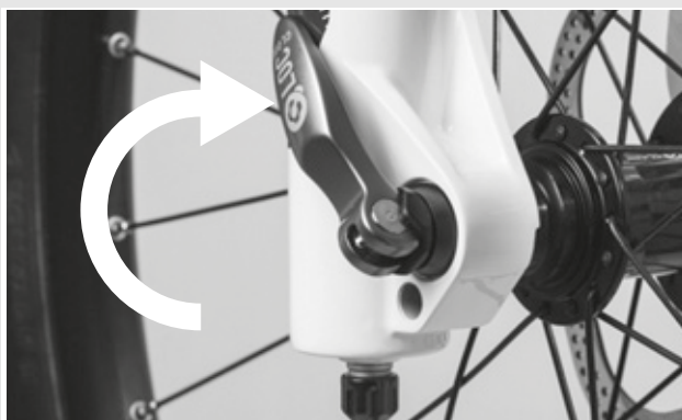
Figure 21: Closing the quick release
