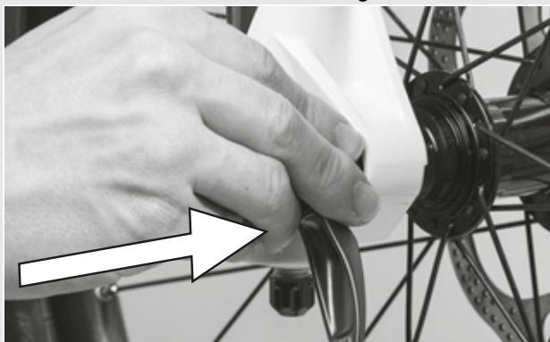
Figure 19: Pushing the quick release in
